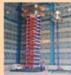
2400kV, 240kV Impulse Voltage Generator
