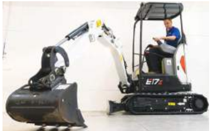
The ZHS functionality on the E17Z facilitates 320° of free rotation when working close to walls and other obstructions. (Photo: Bobcat)
