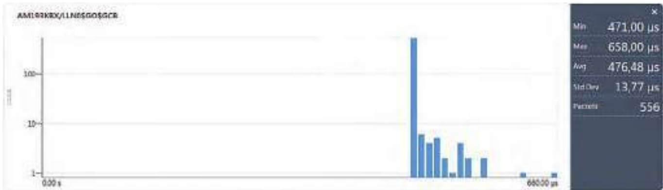
Figure 4: The results of the Propagation Delay Analysis (PDA) run with the DANE0 400 as a worst case scenario were then displayed as a histogram, which shows the delay times for the redundant path.
