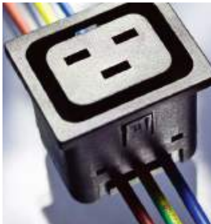
The 4710 is a J style outlet, rated 20 A at 250 VAC by UL/CSA and 16 A at 250 VAC by ENEC.
