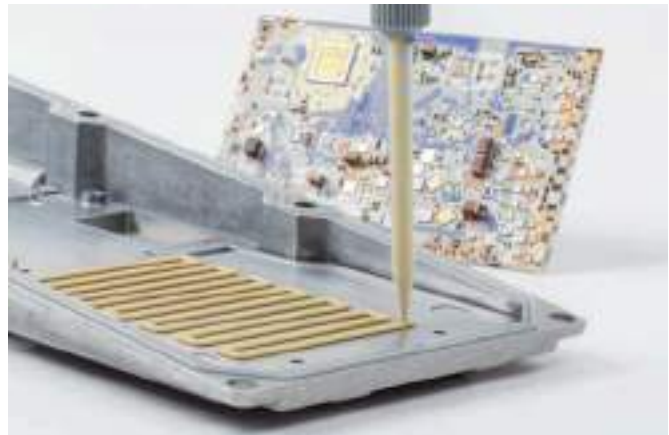
According to the manufacturer, this silicone rubber is an ideal interface material for thermally connecting electronic circuits, ensuring effective heat management. (Image Source: Wacker Chemie AG)
